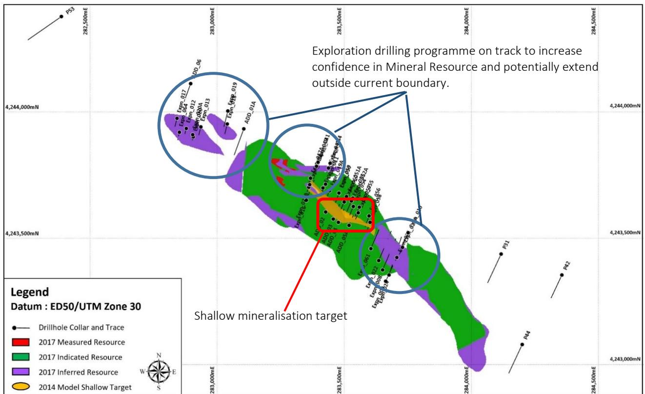
Figure 2. Oropesa geological resource depicting the diamond drilling program and proposed diamond drill hole locations.
