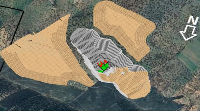
Figure 5: The pit shell and waste location at years 1, 5, 7, 9, 11, and 14 years of operations
