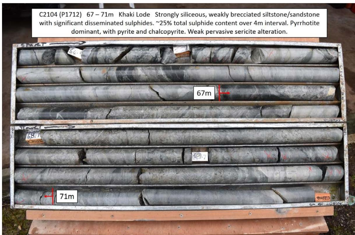
*Drill hole C2104 mineralised zone from 67.1m to 71.0m*
