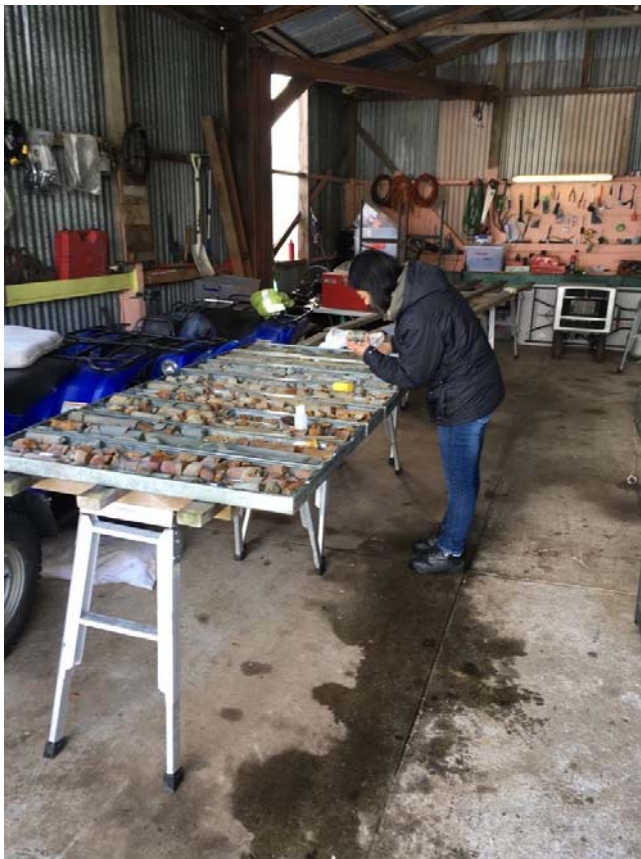
Figure 1. Logging drill core from drill hole C2102
