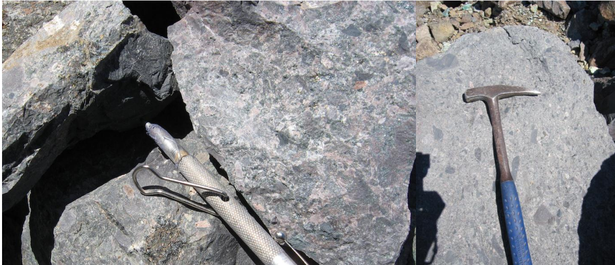
Figure 9: Disseminated sulphide minerals (chalcopyrite, bornite, pyrite) within polymictic hydrothermal breccias.
