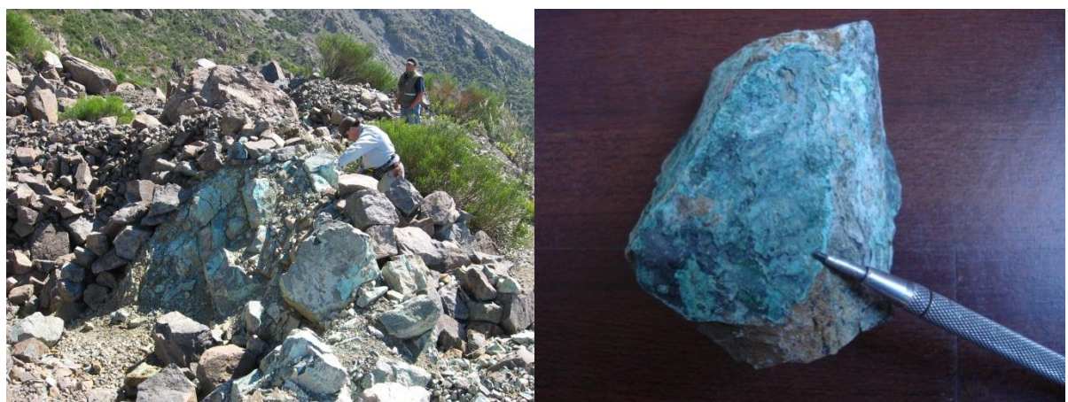
Figure 8: Copper oxide mineralisation in the wallrock mantos.
