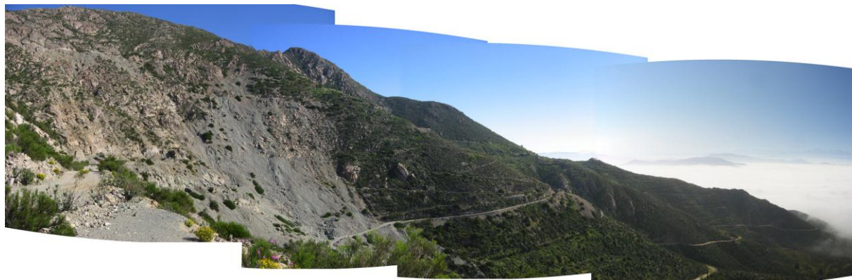
Figure 6: Waste dumps beneath old workings that mantle the eastern flank of Cerro Tamaya in the southern sector. Access roads cut into the hillside indicate that extraction took place on multiple levels.
