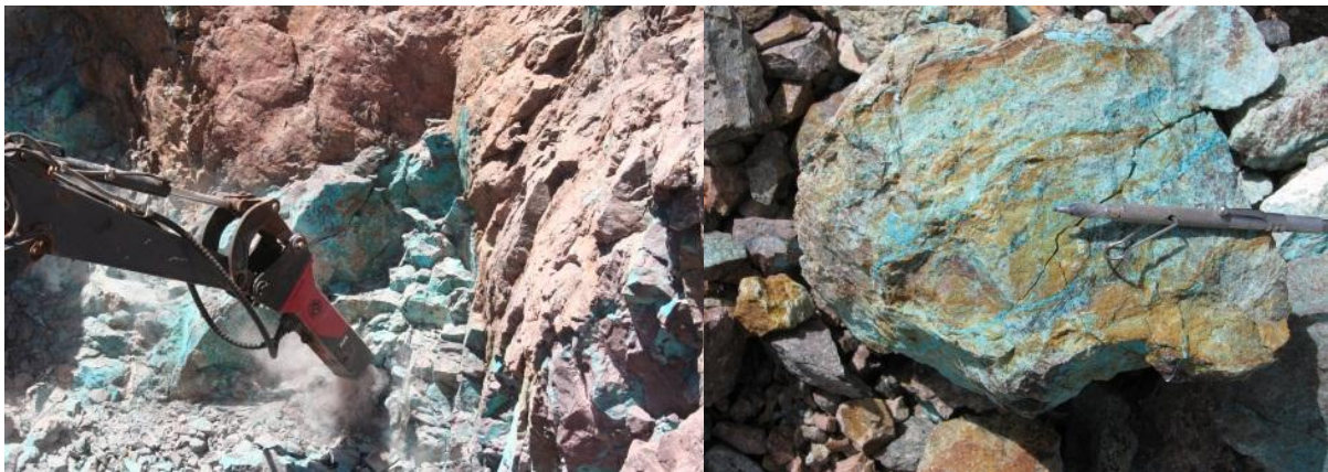
Figure 6: Excavating a newly exposed high-angle structure at Mercedes (left) and an example of high-grade copper oxide mineralisation from the structure (right).
