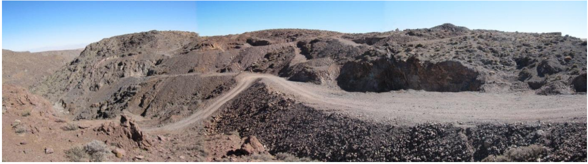
Figure 4: Main Mercedes workings showing mineralisation extending over 400 metres in length and over a vertical extent of 150 metres. A selective sample assayed 3.09% copper and 36 g/t silver.
