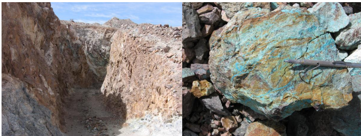
Figure 4: Elvira prospect showing the upper part of the porphyry zone, grey in colour, intruding into the volcanics, red-brown in colour (left) and mineralisation in the porphyry (right).
