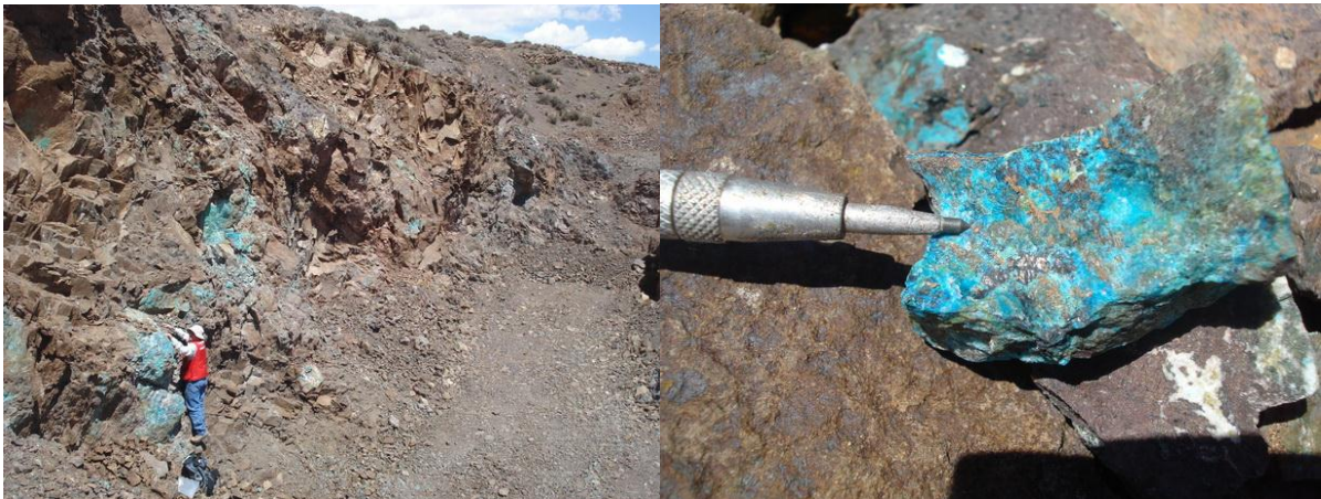
Figure 2: Mineralised manto at Mercedes 1 prospect (left) and a sample assaying 2.65% copper (right).
