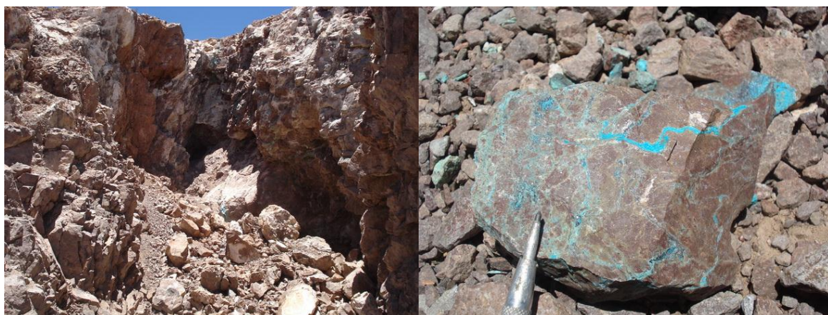
Figure 5: Pamela zone with mineralised fracture zone in volcanics (left) and material forming a sample assaying 9.79% copper (right).
